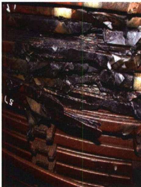
Station 3 Gen Transformer 4 HV winding failure
