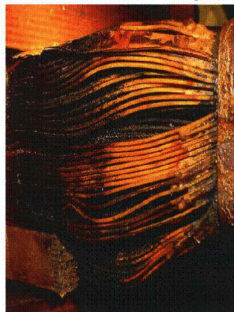
Station 3 Gen. Transformer 5 evidence of overheating
